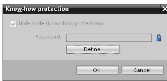
Figure 15-3 Setting up block know-how protection (2)
